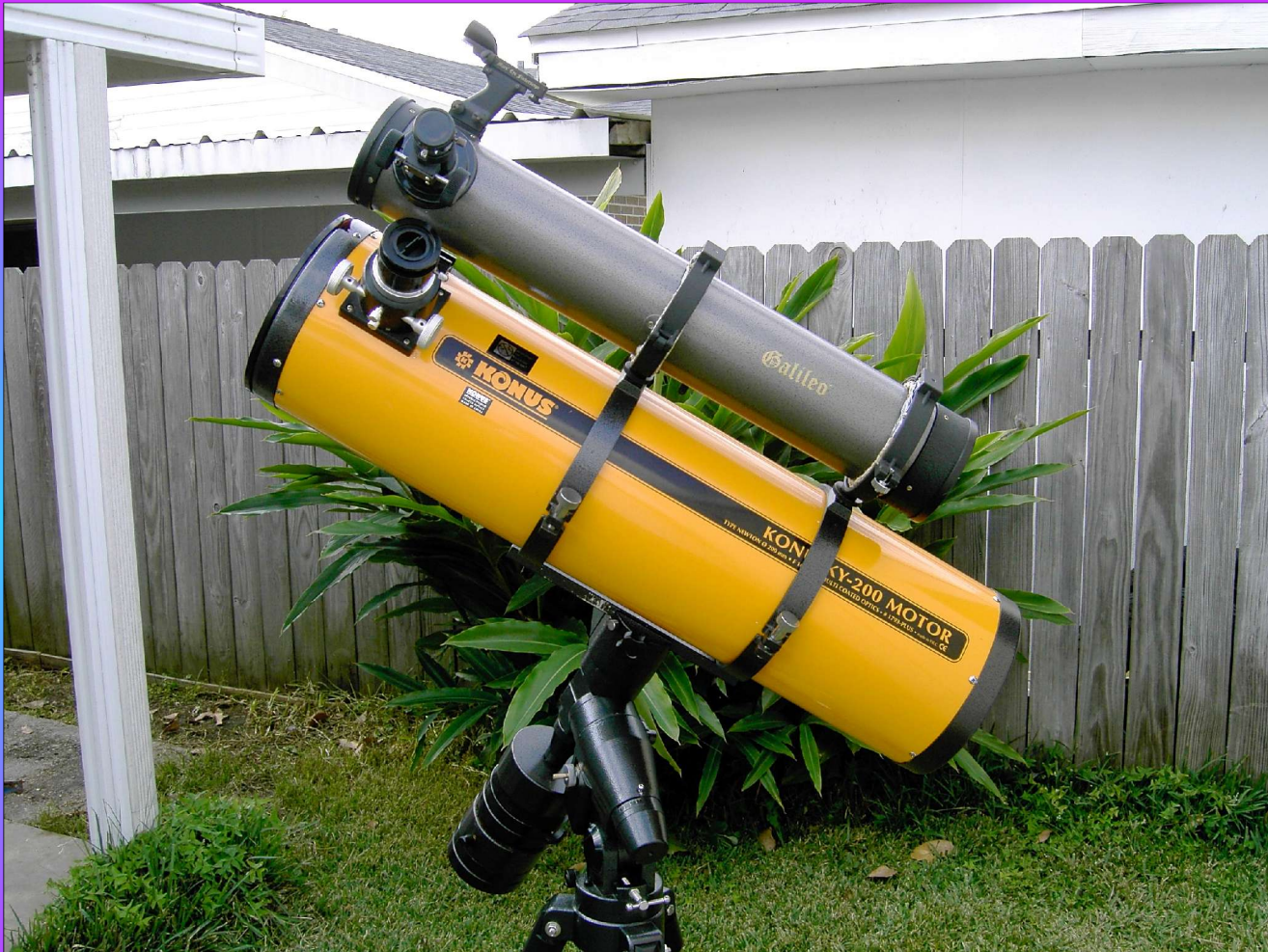
8" Konus f/5 Newtonian Reflector and 80mm guidescope/ finder.
